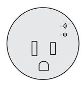
125 V ac. 60 Hz. 15 A Resistive. 15 A General Use, 1000 W Tungsten, 500VA Electronic Ballast. 120 V ac, 60 Hz, 8.3 A Ballast, 1/2 HP
